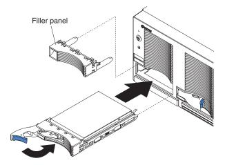
d. Check the hard disk drive status LED to verify that the hard disk drive is operating properly.
